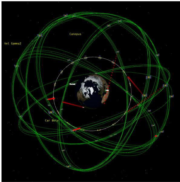
(a) Rendering of a constellation of 16 satellites (white orbit line) with ground stations and GPS satellites (green orbit lines) visibility
