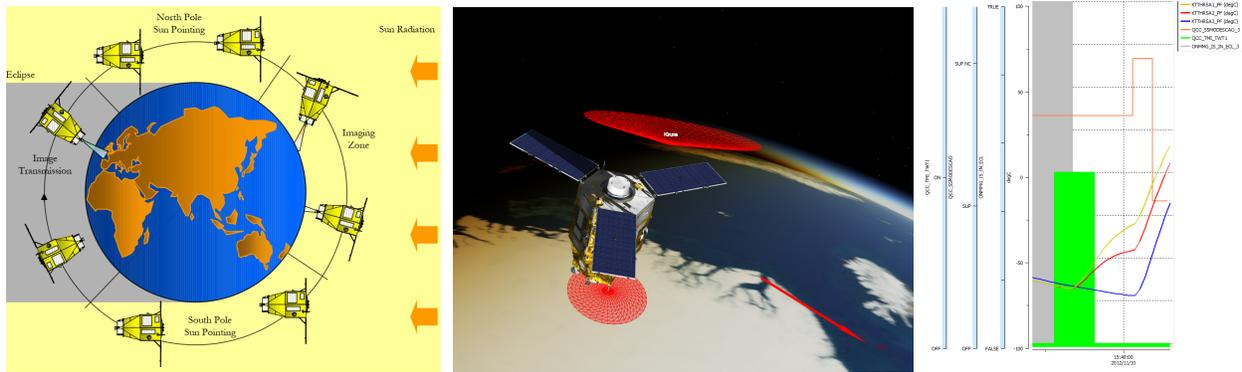
(a) Satellite pointing of Pléiades along the orbit. As the attitude changes often during the short orbit (1h40) a 3D visualization is essential to understand the system behaviour.
