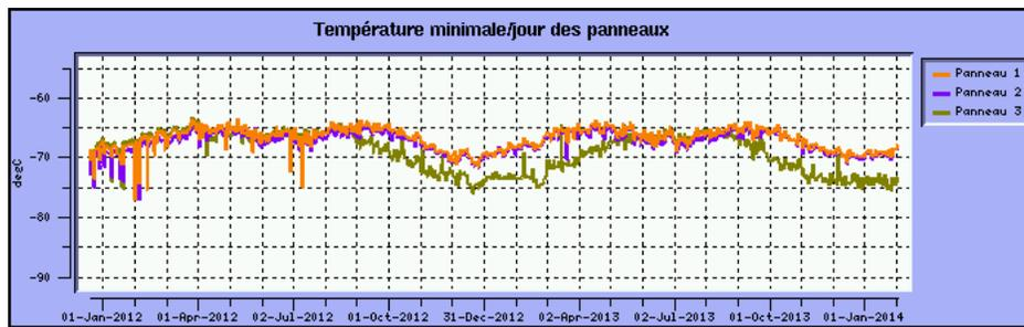
(d) The masking also induces a seasonal variation of the minimum temperature on the shadowed solar array panel (as plotted in green).
