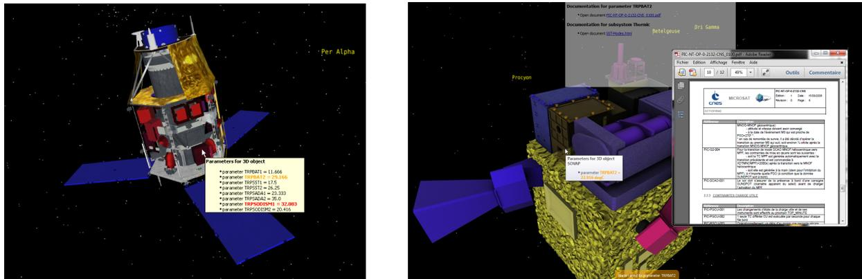
(a) A 3D colour-coded representation for the thermal control of equipment (blue indicates a low temperature and red indicates a high temperature)
