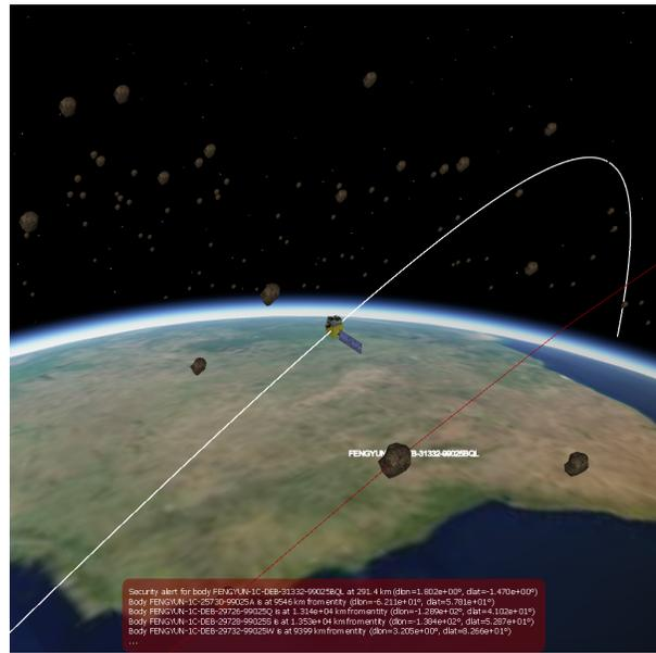
(b) Rendering of a huge set of debris (Fengyun-1C) scaled up to make them visible, the ones nearer than a user-defined distance are highlighted (red orbit line)
