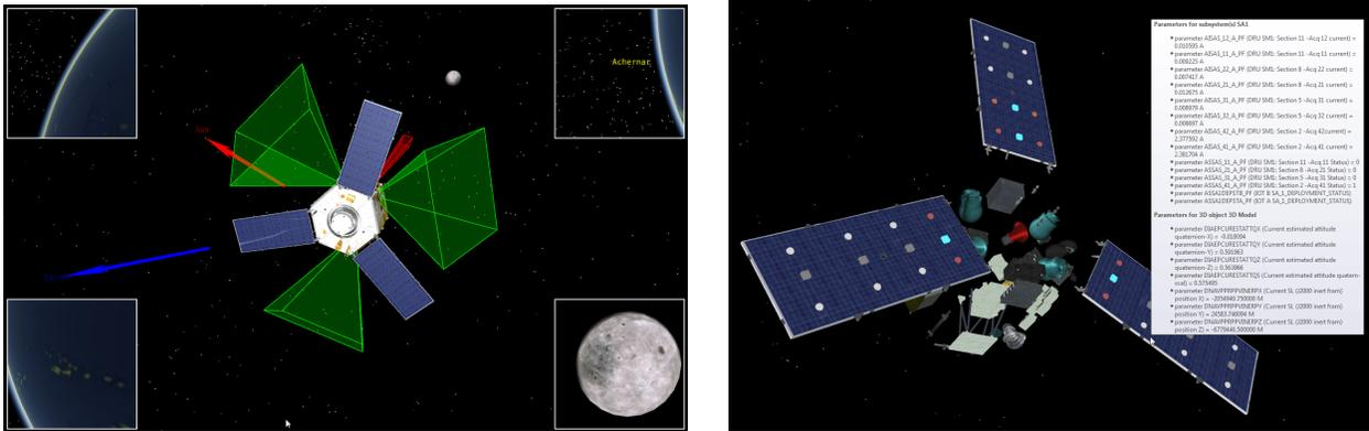
(a) A synthetic picture of all the sensor field of views of Pléiades (star trackers are shown in green and the optical sensor in red). The inserts in the corners simulate the different views from the sensors, where one can see that the star trackers are blind by the Earth while the optical sensor acquire the Moon.
