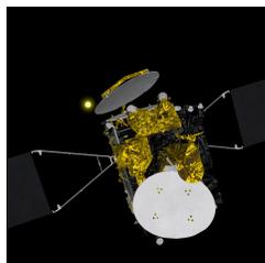
(b) Partially deployed first reflector
