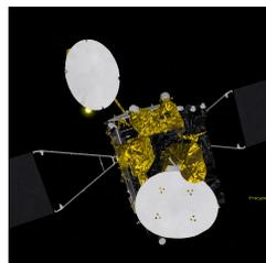
(c) Totally deployed first reflector
